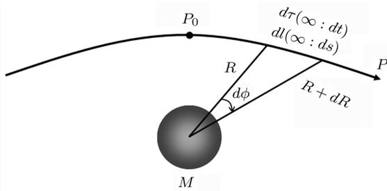
**Fig. 1.** Light deflection caused by a curved spacetime.
