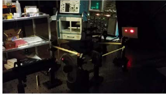
Figure 2.2.1. [Video online] Mechanically blocking any one of the two incident beams on the beam combiner from the opposite sides converts the beam combiner into a regular 50/50 beam splitter. Blocking destroys the emergence of the superposition effect; which is its capability to re-direct 100% of the energy out of the two beams into one of the selected direction, depending upon the phase condition, as the mirror M1 keeps scanning (see Fig.2.1.2).
